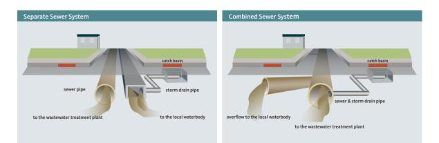
In cities with combined sewer systems, stormwater from streets and wastewater from homes, buildings and industry is collected by a single pipe and is delivered to a wastewater treatment facility. In the event of a heavy flood or snowmelt, a combined sewer system can become overwhelmed with the incoming volume of water. This results in a combined sewer overflow where untreated stormwater and wastewater is discharged directly into nearby streams and rivers.
